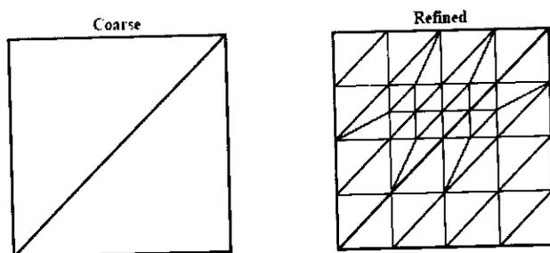
Fig. 2. Subdivision of the triangular cells using adaptive gridding strategy.
