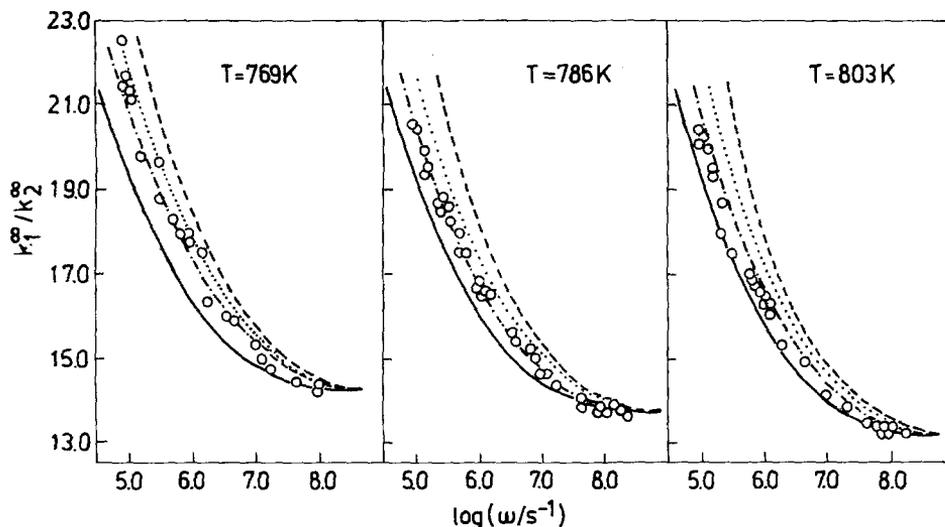
Fig. 3. Pressure dependent ratio of the two reaction channels for TFCB decomposition at 769, 786 and 803 K. O Experimental; (—) RRKM strong collision hypothesis; (---) RRKM stepladder model with  $\langle \Delta E \rangle_d = 1200 \text{ cm}^{-1}$ ; ( $\cdots$ )  $\langle \Delta E \rangle_d = 1500 \text{ cm}^{-1}$  and (-·-)  $\langle \Delta E \rangle_d = 1800 \text{ cm}^{-1}$
