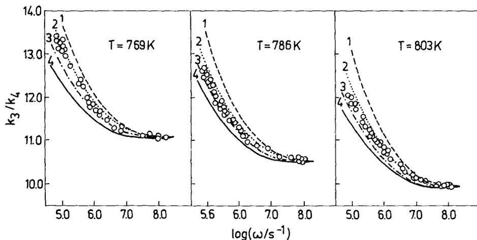
Fig. 4. Pressure dependent ratio of the two reaction channels for MTFCB decomposition at 769, 786 and 803 K.  $\circ$  Experimental; (—) RRKM strong collision hypothesis; (--) RRKM stepladder model with  $\langle \Delta E \rangle_d = 1200 \text{ cm}^{-1}$ ; ( $\cdots$ )  $\langle \Delta E \rangle_d = 1500 \text{ cm}^{-1}$  and (-·-)  $\langle \Delta E \rangle_d = 1800 \text{ cm}^{-1}$
