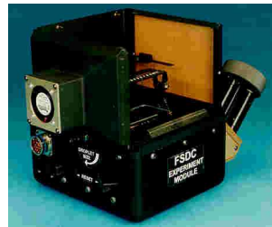
FSDC: Fiber-Supported Droplet Combustion burning of methanol droplets, fixed by glass fibers
