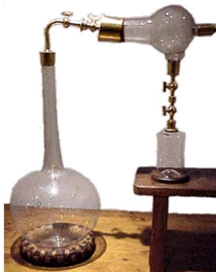
the original apparatus of Lavoisier
