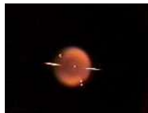
FSDC: Fiber-Supported Droplet Combustion burning of methanol droplets, fixed by glass fibers
