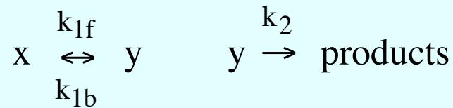
$$\frac{d}{dt} \begin{bmatrix} X \\ Y \end{bmatrix} = \begin{bmatrix} -1 \\ +1 \end{bmatrix} (X - Y) + \begin{bmatrix} 0 \\ -1 \end{bmatrix} \frac{Y}{\varepsilon} \quad \varepsilon = 10^{-6}$$
