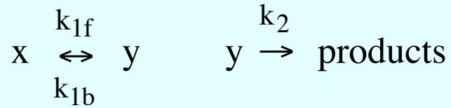
$$\frac{d}{dt} \begin{bmatrix} X \\ Y \end{bmatrix} = \begin{bmatrix} -1 \\ +1 \end{bmatrix} \left( X - \frac{Y}{\varepsilon} \right) + \begin{bmatrix} 0 \\ -1 \end{bmatrix} Y \quad \varepsilon = 10^{-6}$$
