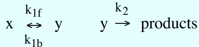
$$\frac{d}{dt} \begin{bmatrix} X \\ Y \end{bmatrix} = \begin{bmatrix} -1 \\ +1 \end{bmatrix} \left( \frac{X}{\varepsilon} - Y \right) + \begin{bmatrix} 0 \\ -1 \end{bmatrix} Y \quad \varepsilon = 10^{-6}$$
